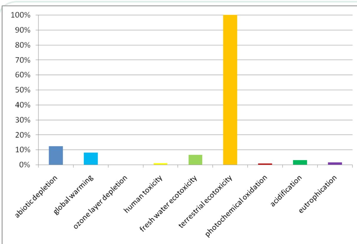
**Figure 3. Normalized results per impact category of a school desk made from FSC certified wood (based on data from Gonzalez et al., 2008).**
