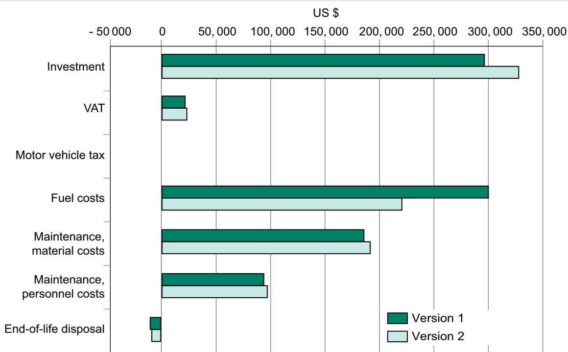
Figure 7. LCC of standard public transport heavy duty bus (in US\$) (adapted from Ruedenauer et al. 2007).
